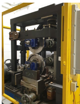
Figure 6: A photograph of the twin disc testing machine at the IRR.
