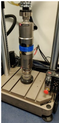
Figure 5: A photograph of the Instron 8874 tensile testing machine used in this study.
