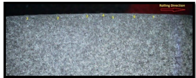
Figure 16: A 100 x magnification photograph showing RCF cracks on a R260 sample subjected to RCF twin disc conditions.
