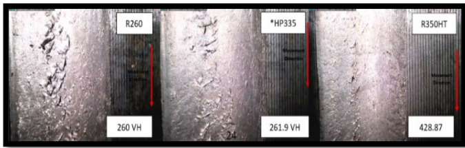
Figure 14: An illustrated compilation of 200x magnification photographs showing cracks and damage (Test 1).
