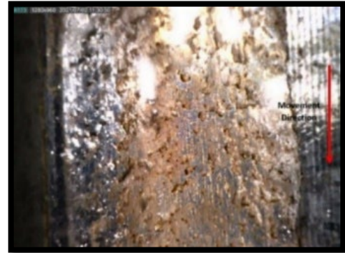
Figure 1: A 200x magnification photograph of a wet rail sample surface.
